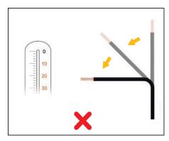
No bending at low temperatures (< 0°C or < 30F)
