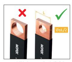
Do not drill holes exceeding half of the width of the bar
