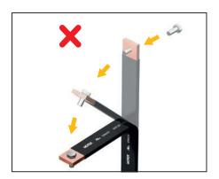
Copper files slide when bending to compensate the different length of inner and outer file
