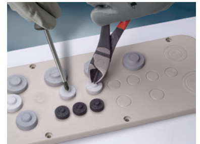
Make a small hole into the membrane using a screwdriver or cut the top of the cone using side cutters.
