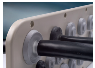
(Front side) Pull the cable or tube back for some 20 mm to lock it.
