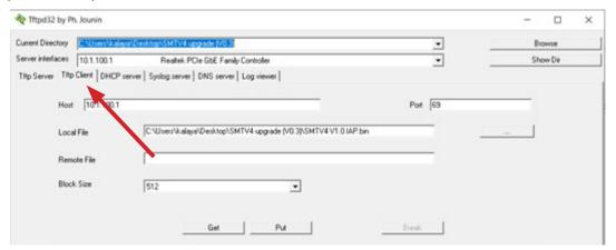
Step 2: Select PC IP address, for example the PC side IP address is 10.1.100.1
